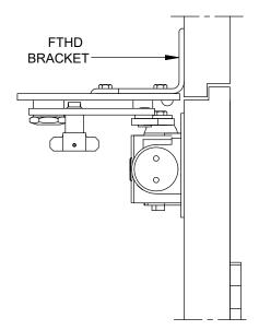
DOOR CLOSER MODELS: 8916, 8956 SPA, SPAT, SPAK x FTHD PARALLEL ARM INSTALLATION (PUSH SIDE MOUNT)
