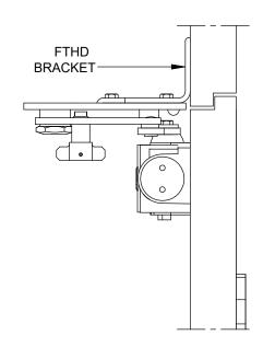
DOOR CLOSER MODELS: 8916, 8956 SPA, SPAT, SPAK x FTHD PARALLEL ARM INSTALLATION (PUSH SIDE MOUNT) FLUSH TRANSOM BRACKET
